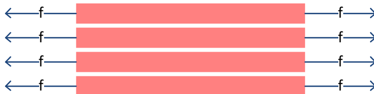
Figure 2 Force Distribution on a Straight Rope
