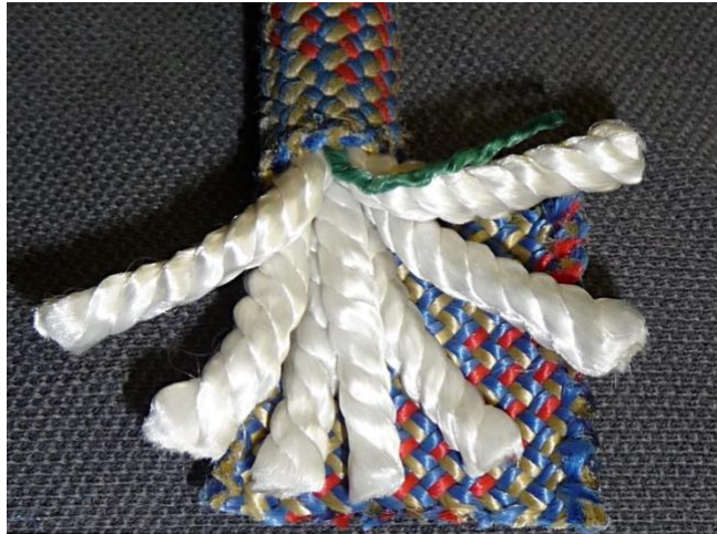
Figure 1 Construction of a Kernmantle Rope
